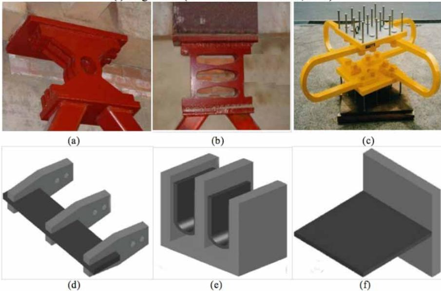
dampers (e.g. X-shaped, single round-hole, U-strip, torsional beam, tapered cantilever, single axis and steel panel-based) have been proposed in accordance with place of use, ease of installation and type of frame structures.
